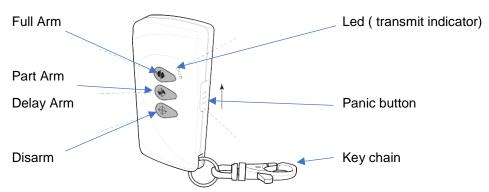
The Remote Control incorporates a Personal Attack Switch (Panic). Activating the Panic Alarm will immediately initiate a Full Alarm condition whether the system is Armed or Disarmed, (unless the system is in Service, Test or Program mode).
